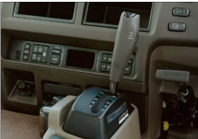
6 spd AISIN automatic transmission
